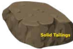
Hardened tailings are compact, strong and can stand on their own. A sample of 7,6cm (3in) in diameter by 25,4cm (10in) long can withstand 6kg (13lb) of weight stacked on it.
